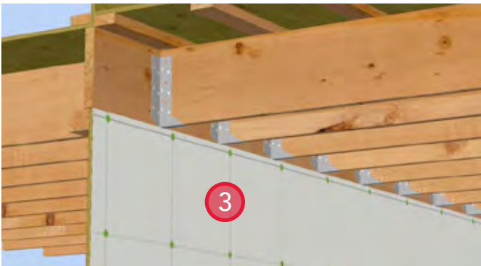
3. Install sheathing membrane and apply pressure to ensure adhesion to the acoustical sealant bead.
