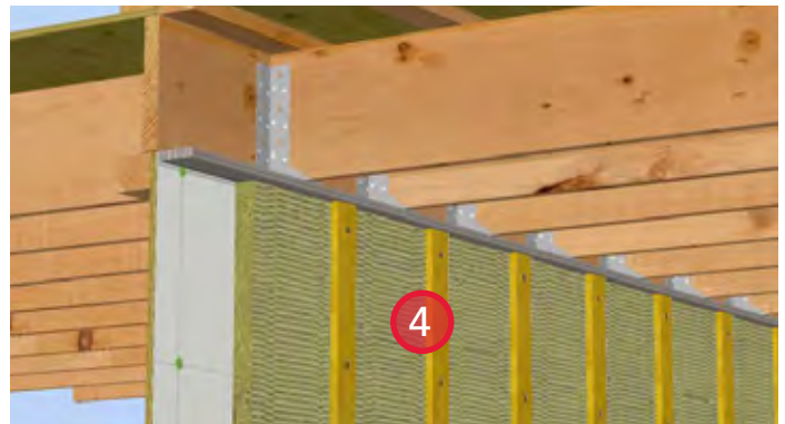
4. Install ROCKWOOL COMFORTBOARD™ 80 and strapping with bugscreens, leaving a \frac{3}{4} " gap to ensure air barrier continuity through sheathing to rim joist interface. Suggest using a 1x4 temporary spacer board to space the insulation.
