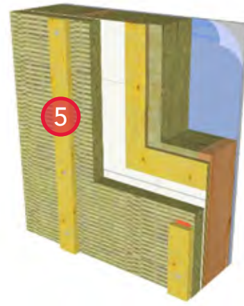
5. Install CAVITYROCK® and secure with strapping.
