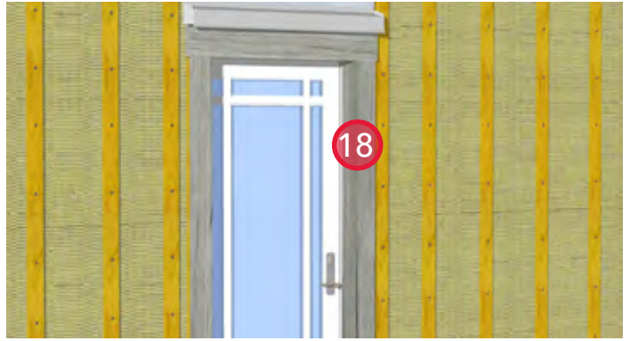
18. Install swing door trim boards.
