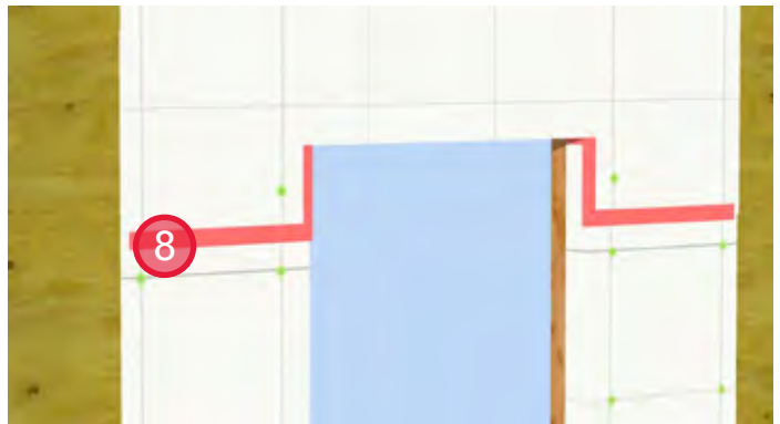
8. Install sheathing tape at the leading edges of the sheathing membrane to maintain air barrier continuity.
