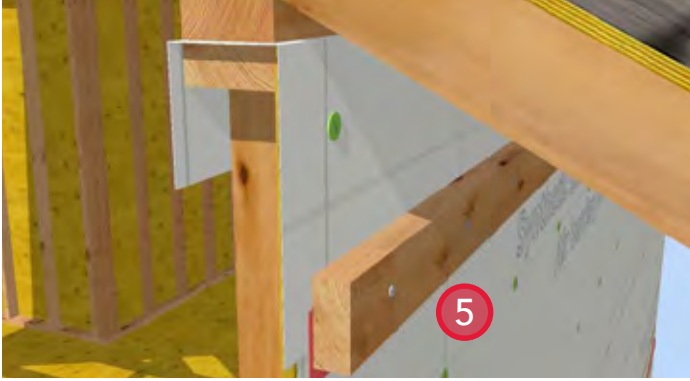
5. Install a 2x4 ledger board to support the soffit material and venting.
