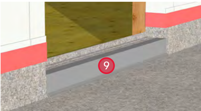
9. Install sub-sill prefinished metal flashing. Adhere to the PVC deck membrane to avoid puncture of the membrane.
