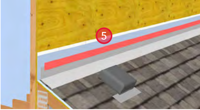
5. Install a metal closure flashing and seal the leading edge with sheathing tape to the waterproof membrane, to provide for air barrier continuity.
