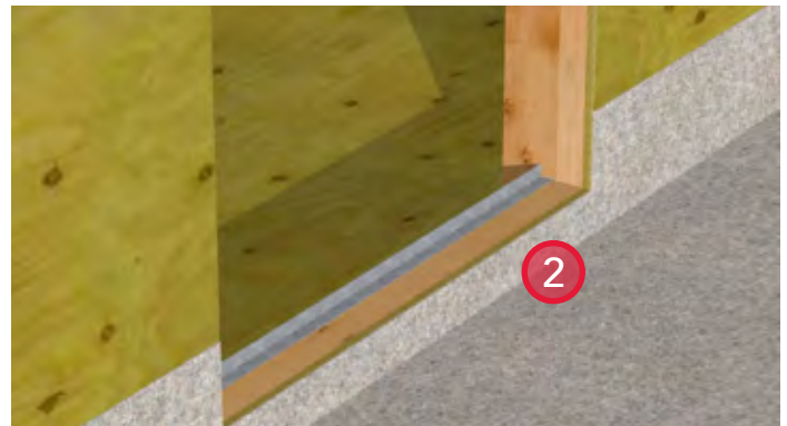
2. Install PVC balcony membrane. Extend the membrane to the height of the rough opening and elsewhere to a minimum height of 8" above the finished deck grade.
