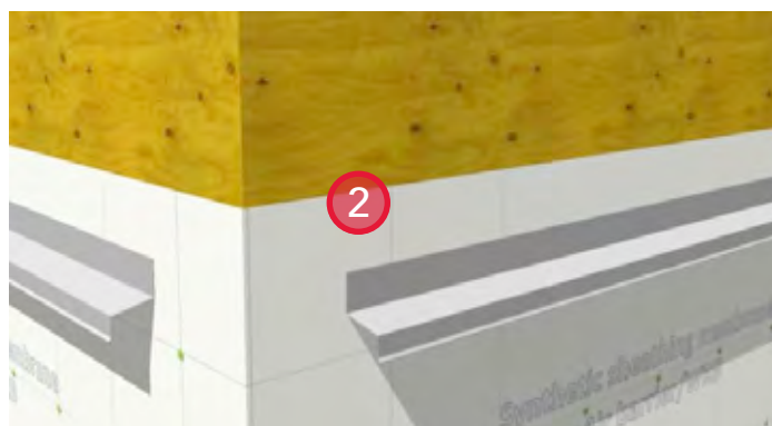
2. Install sheathing membrane and flashing.
