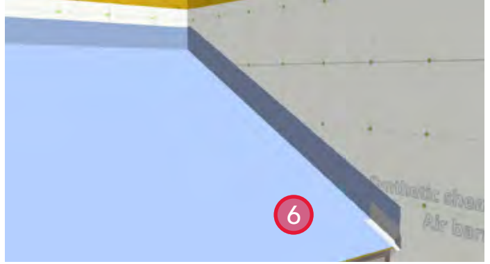
6. Install first step of the stepped flashing with a kickout to divert water towards the gutter and away from the adjacent wall.
