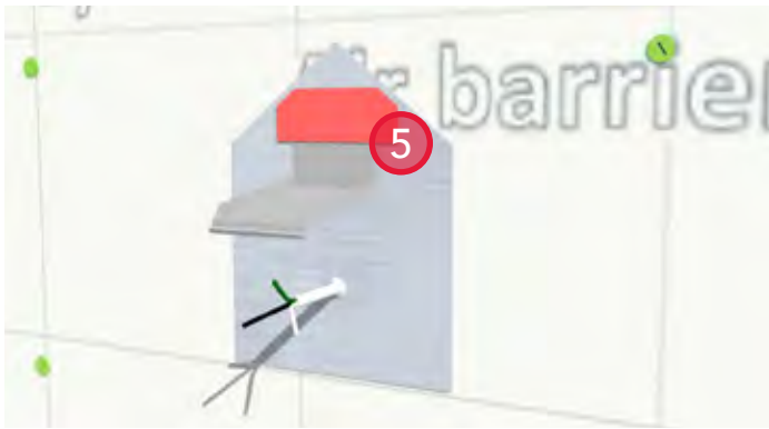
5. Install prefinished metal flashing over the penetration and seal with sheathing tape to provide for air barrier continuity.
