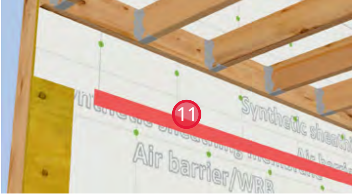
11. Install sheathing membrane below the canopy. Ensure the membrane laps under the starter strip. Seal the leading edge of the starter strip membrane with sheathing tape to maintain air barrier continuity.
