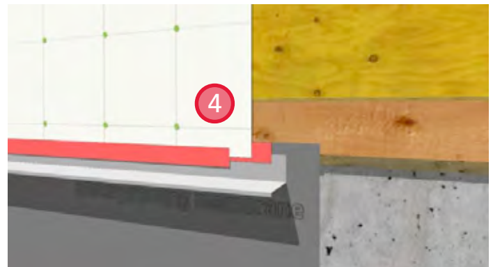
4. Install sheathing membrane and seal leading edge to the flashing with sheathing tape to complete air barrier continuity. Provide a \frac{3}{4} " vision line on the flashing backleg.
