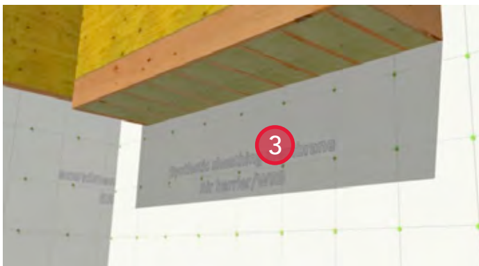
3. Install sheathing membrane. Cut to allow the membrane beside the cantilevered floor to extend up the wall 8".
