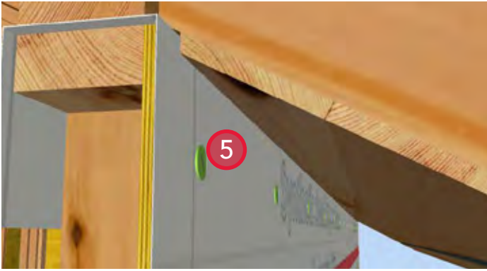
5. Install soffit material and vents.
