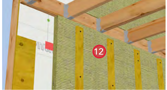
12. Install ROCKWOOL COMFORTBOARD™ 80 and secure in place with strapping. Provide bugscreens at the top and bottom of the strapping.
