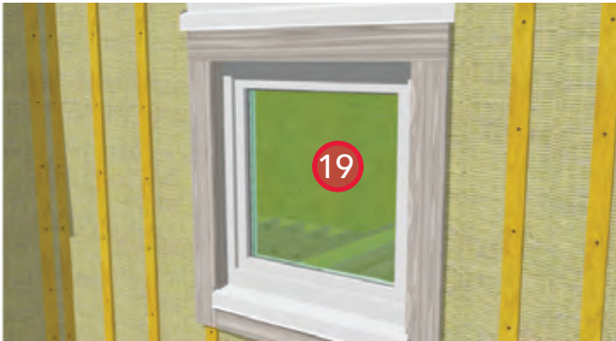
19. Install metal flashing to the strapping over the top window trim board.
