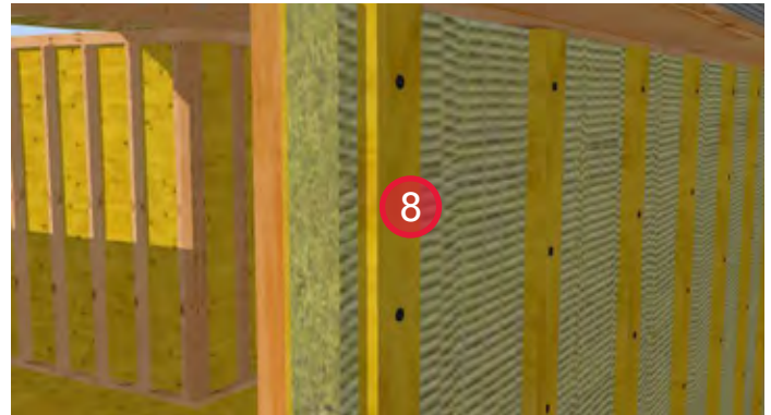
8. Install ROCKWOOL COMFORTBOARD™ 80 and strapping. Provide bugscreens at the top and bottom of the strapping.
