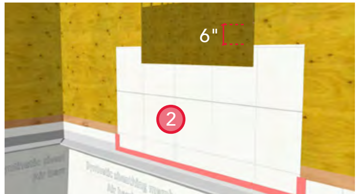
2. Install starter strip of sheathing membrane below the window rough opening. Seal the leading edge with sheathing tape.
