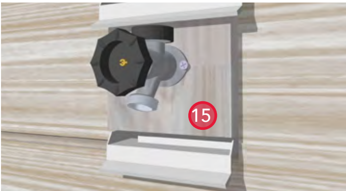
15. Install the cladding.
