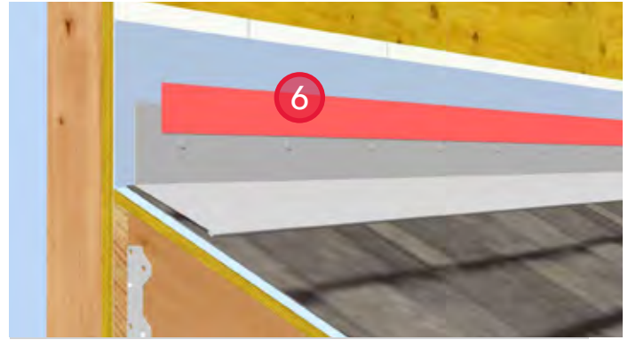
6. Install prefinished metal closure flashing and seal the leading edge with sheathing tape to provide for air barrier continuity.
