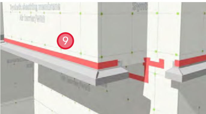
9. Seal the leading edge of the sheathing membrane with sheathing tape to maintain air barrier continuity.
