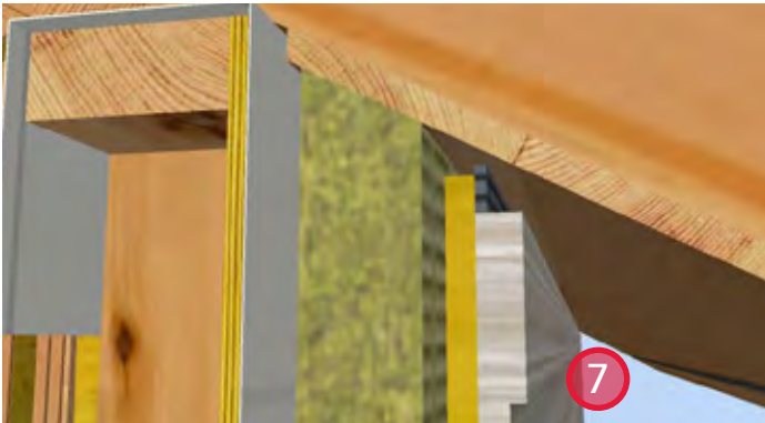
7. Install cladding. Allow for venting of the wall cavity at the top of the cladding underside of the soffit.
