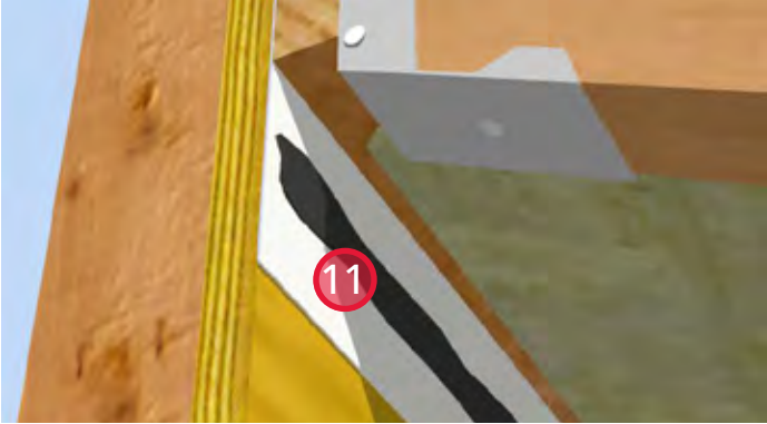
11. Apply a bead of sealant to the exterior of the sheathing membrane for air barrier continuity.
