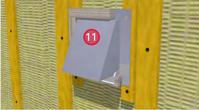
11. Install cladding and trim boards around the exhaust vent hood.
