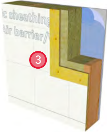
3. Install sheathing membrane.
