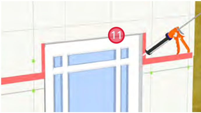
11. Install backer rod and sealant around the exterior perimeter of the door frame.
