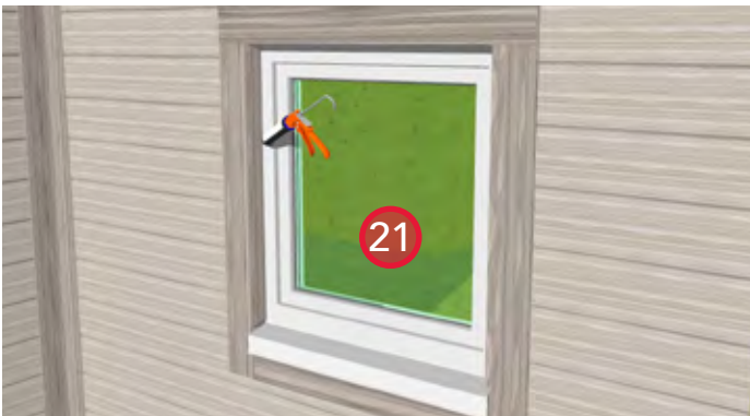
21. Apply sealant around the perimeter of the window (top and sides) between the frame and the window trim boards.
