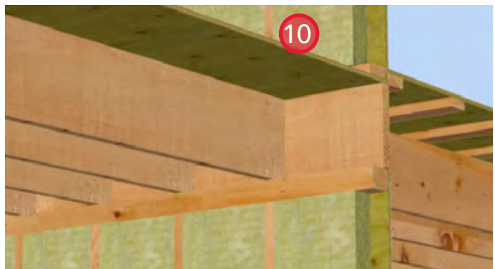
10. Install ROCKWOOL COMFORTBATT® in the interior stud cavities.
