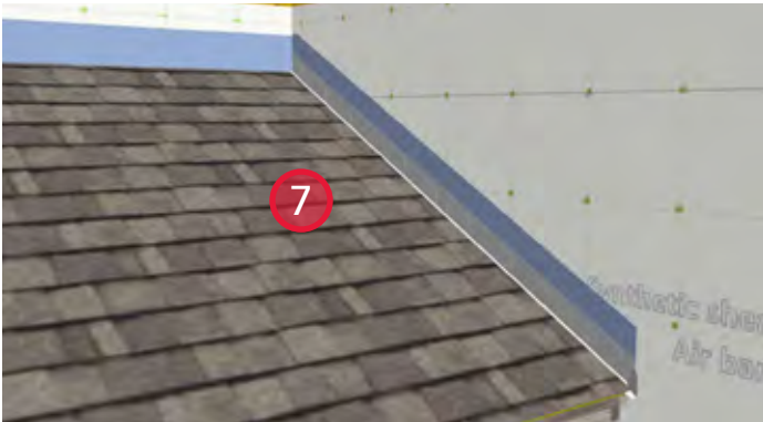
7. Install step flashing and shingles.
