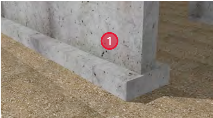
1. Intersection of the concrete foundation wall with the footing.
