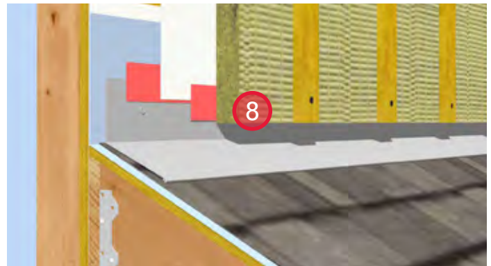
8. Install ROCKWOOL COMFORTBOARD™ 80 and secure in place with strapping. Provide bugscreens at the top and bottom of the strapping.
