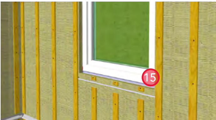
15. Install ROCKWOOL COMFORTBOARD™ 80 and secure with strapping. Provide bugscreens at the top and bottom of the strapping.
