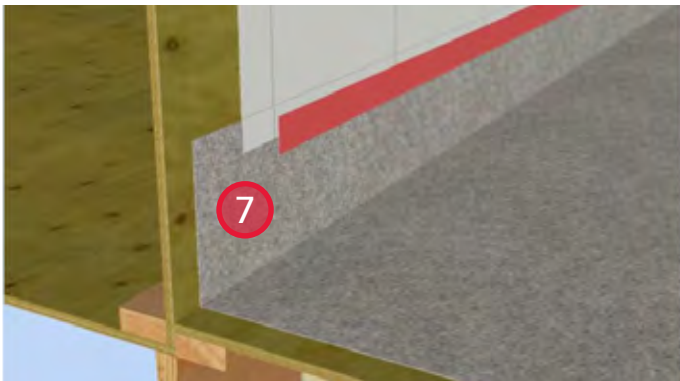
7. Install sheathing membrane and seal the leading edge to the balcony membrane with sheathing tape to maintain air barrier continuity.
