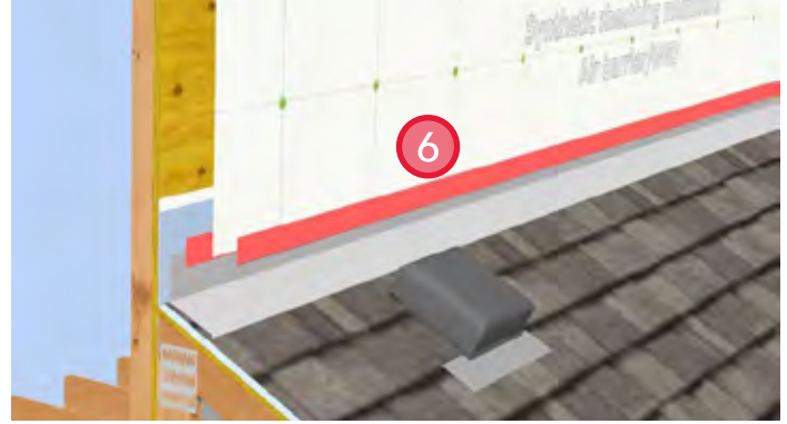
6. Install sheathing membrane and lap over the metal flashing. Seal the leading edge with sheathing tape to complete the air barrier continuity.
