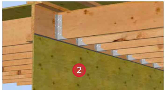
2. Install a bead of sealant along the sheathing directly below the balcony joists to provide for air barrier continuity.
