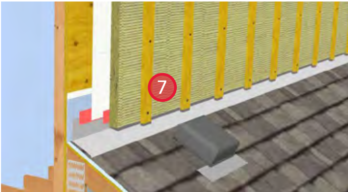
7. Install ROCKWOOL COMFORTBOARD™ 80 and secure with strapping. Provide bugscreens at the top and bottom of the strapping.
